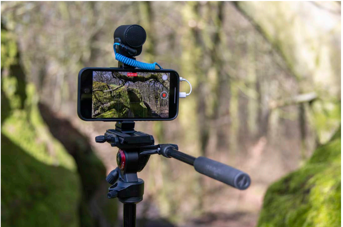
Figure 6, This is the setup I use for videos. An iPhone connected to a Sennheiser MKE 200 directional microphone on a Manfrotto BeeFree tripod. For narration I use a Rode SmartLav+ lapel microphone rather than the Sennheiser.
