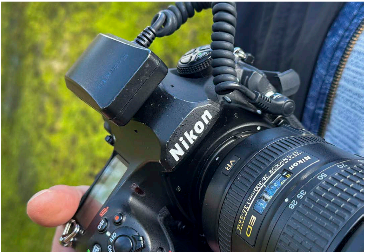
Figure 2. The Solmeta Geotagger GPS attached to a Nikon DSLR. These are great little devices. However, please remember that you will need one specifically designed for your camera.
